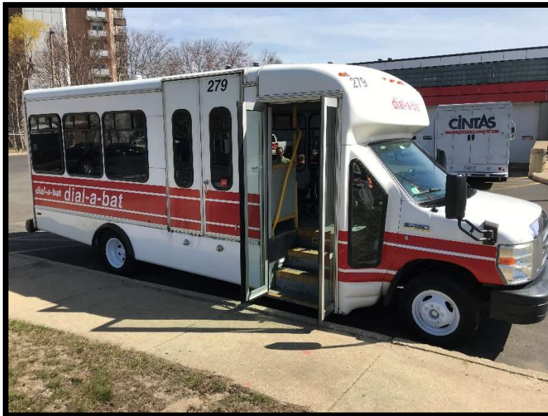
The decommissioned Dial-A-BAT Bus is a 2009 Ford Starcraft E450SD. 25 feet, 8 cylinder, 4 doors, 6 wheels, wheelchair lift. Gross vehicle weight is approximately 14,500 pounds.
