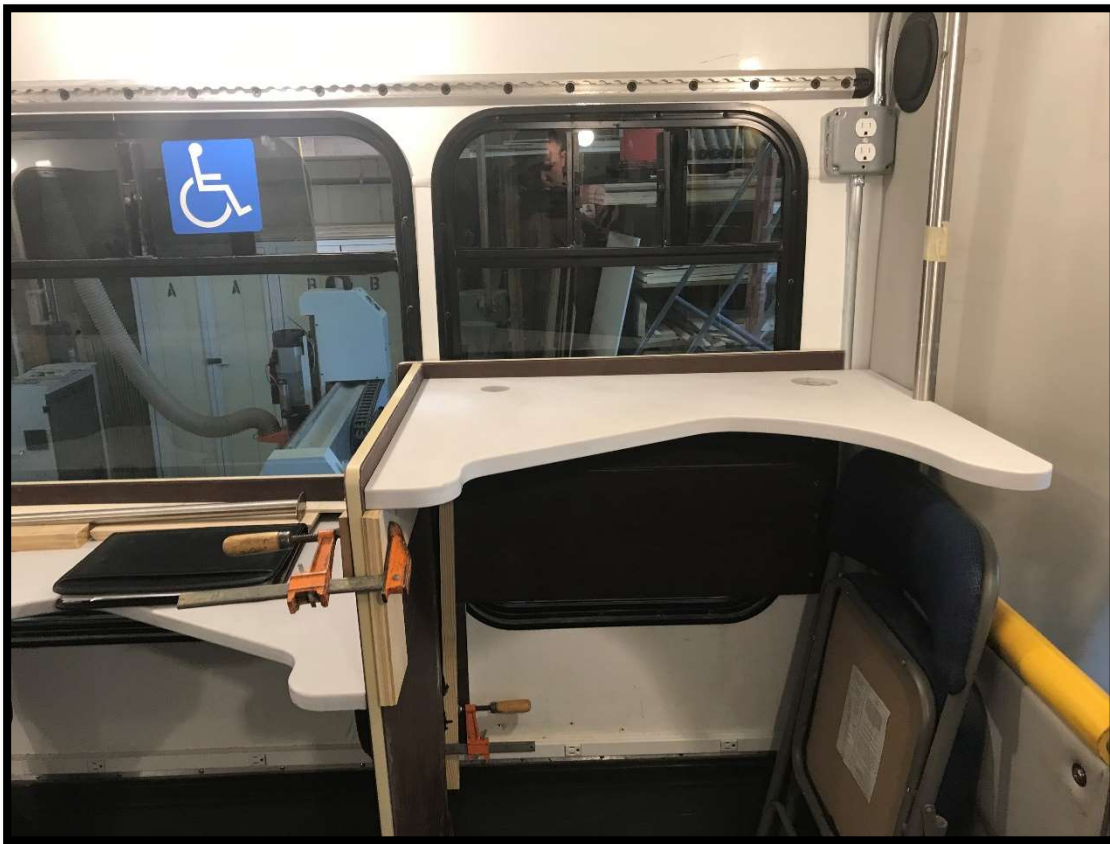
1 chest-level workstation at the front of the vehicle is dedicated for an instructor.
